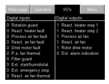
Fig. 3: Status display digital inputs and outputs
