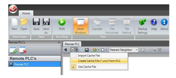
Now, a live connection can be established. To start the remote operation, press <RUN>. The PLC can now be operated remotely.
