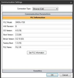
Press <Check Connection> and if the parameters are correct, the PLC information will be shown. Press **<OK>** to confirm.
