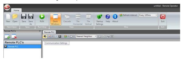
Enter the communication parameters. The PLC name is PLC-35 for unit sizes DA 500 up to DA 4000 and PLC-45 for unit sizes from DA 4400.
